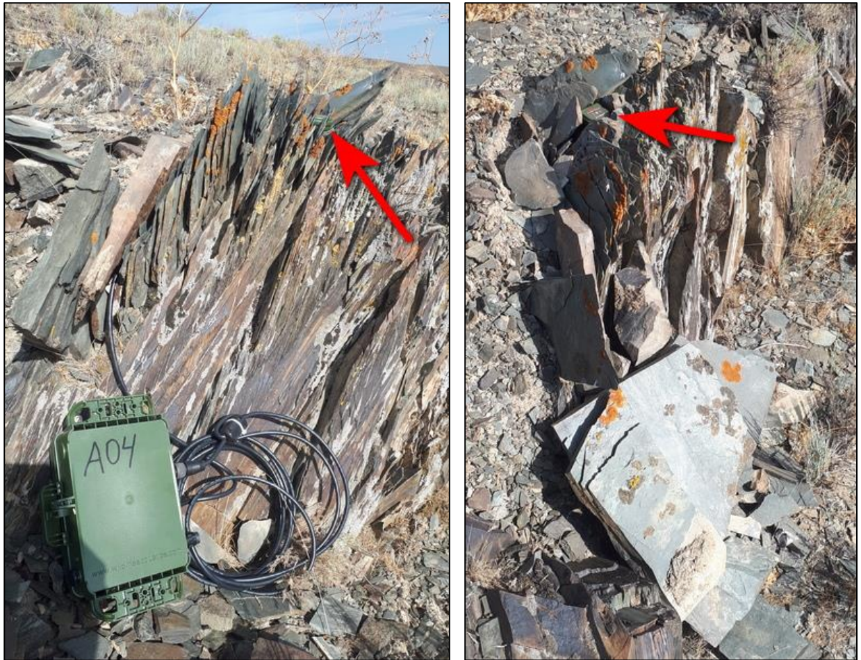
Fig. 11. A variant of hidden placement of a microphone (marked with a red arrow) of a stationary detector in stones on mountain slopes (on the left - before the detector was masked by stones, on the right - after masking).
