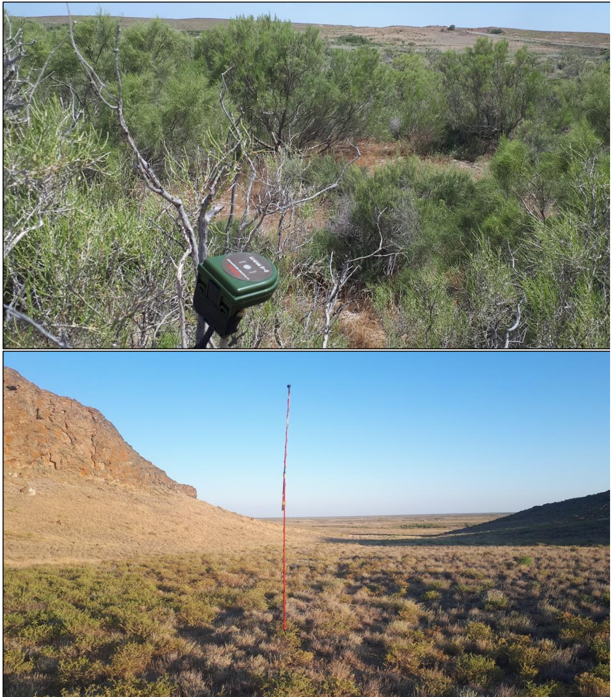
Fig. 10. Options for placing microphones of stationary detectors outside the mountain slopes (above - the detector microphone is fixed on the top of a small tree; below - the microphone is raised on telescopic stands 2-5 m high).
